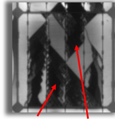
Electroluminescence image showing electrically isolated cell sections
